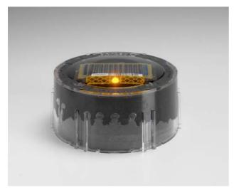
Each unit weighs 470g and is cylindrical, with a diameter of 108mm and a depth of 48mm. The installation engineers simply cut the appropriate size hole in the road surface and anchor of the stud flush to the road surface. As a unit with less than a 4mm protrusion above the road surface, the stud will not be damaged by road maintenance such as snow-ploughing and doesn't present a hazard to cyclists or motor cyclists.
