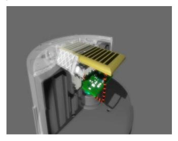
The units can be specified either as bi-directional units with two LEDs and reflectors pointed in opposite directions for use on highway centre-marking, or can be uni-directional, with a single LED, either in amber, white, red or green to meet specific highway marking requirements.
